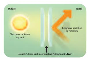
Windows incorporating Pilkington **K Glass**<sup>™</sup> allow heat from the sun through and reflect heat from fires and radiators back inside, making it easier to keep houses warm.
